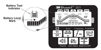
The Receiver batteries are tested for two seconds every time the unit is turned on. The time interval can be extended by pressing and holding On During the battery test, the bar graph should extend to the right of the battery level mark, otherwise replace the batteries.
